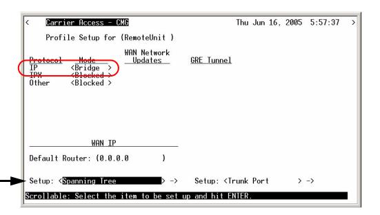
4. To enable Spanning Tree, scroll **<Disabled>** to **<Enabled>**, with the **[SPACEBAR]**, select **[ENTER]**.
